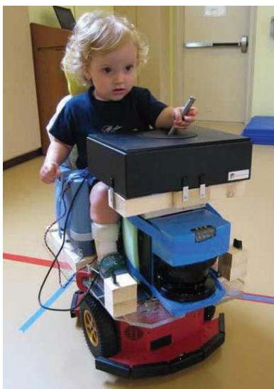
Pediatric mobile robots help children learn how to navigate using force-feedback joysticks.
